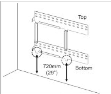
2. Mount the wall bracket to a wall. Tighten the screws, ensuring that they are horizontally driven into the wall. (Must be installed with recommended clearances(720mm[29"]) on the edge of the wall bracket as shown in the figure)
