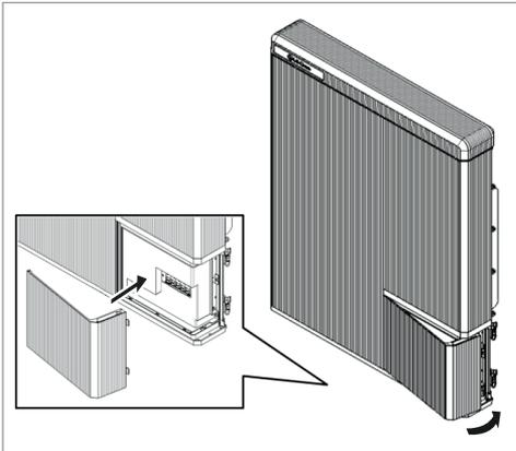
5. Close the transparent protection cover and tighten the screw. (Marked position)
