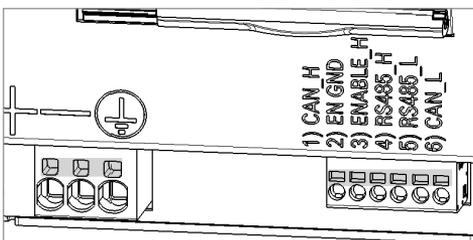
1. To remove one of the wires from its terminal, insert a small screwdriver into the rectangular hall above the terminal.
