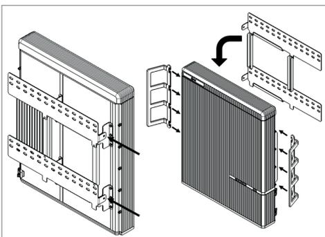
9. Loosen the two hex-socket screws using a socket wrench to detach the battery pack from the wall using lift handles.
