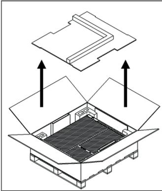
3. Remove the wall bracket guide pad & cushioning pad.
