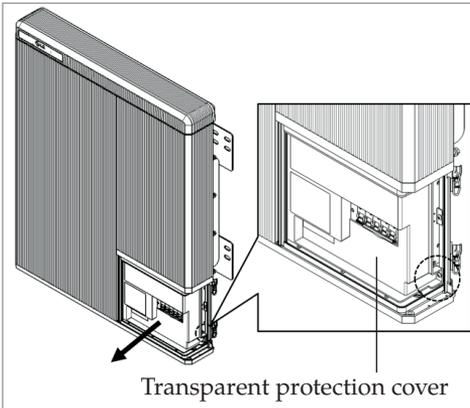
7. Loosen the screw (marked position), and remove the transparent protection cover.
