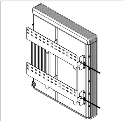
4. Tighten the two hex-socket screws enclosed and remove the lift handles. The nuts for these screws are welded to the battery pack chassis. Tighten to a torque of 5 N·m using the M6 torque wrench.
