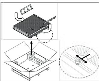
5. Pull out the battery pack using handles and stand it up.
