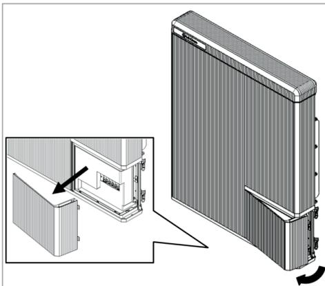
3. Open the wiring box cover (about 2~10 degrees), and pull to remove it.
