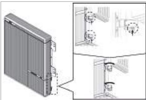
5. Press the two buttons and pull the two latches (marked position) on the rear side of the wiring box cover (hinged door).
