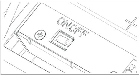
4. Auxiliary power ON/OFF switch (for shipping and storage)
