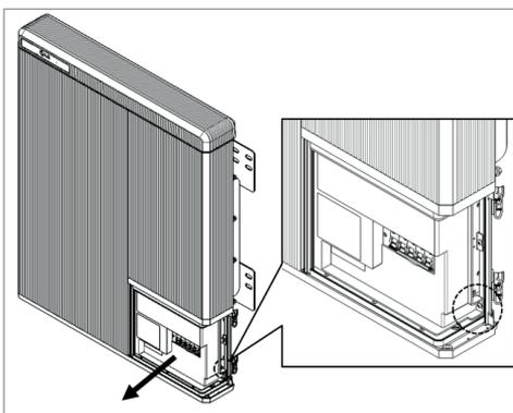
4. Loosen the screw (marked position), and remove the transparent protection cover.
