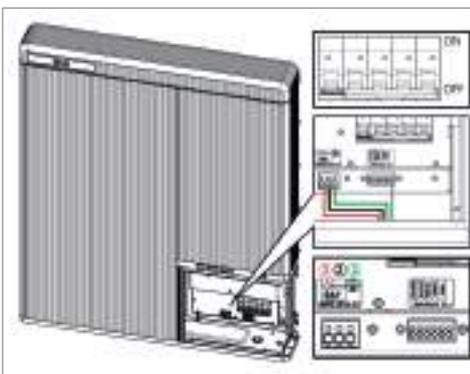
9. Connection Power / Communication cables, according to the labels marked.
