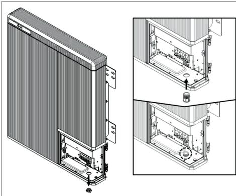
8. Remove the cap on hole in the bottom side, and assemble the 3/4" conduit plug. In the case outdoor, it must be sealed to comply "IP55" [ex) gasket, sealing foam, silicon, etc], where the battery pack installation is outdoor.
