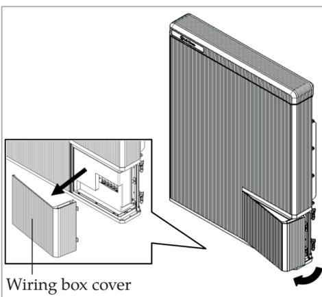
6. Open the wiring box cover (about 2~10 degrees), and pull to remove it.
